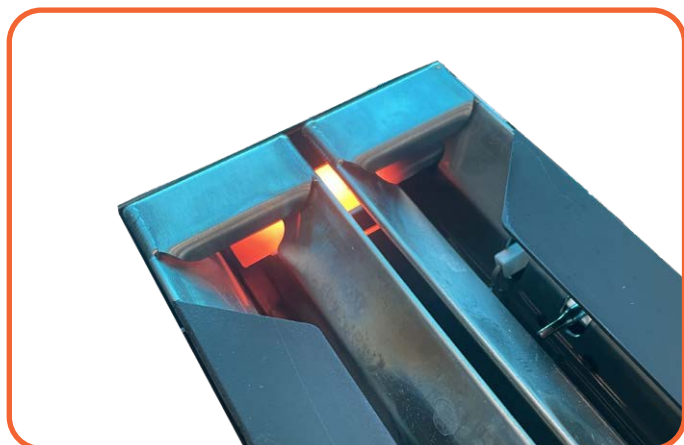
Figure. 4.5 PRIMING: Fuel is going to be ignited
